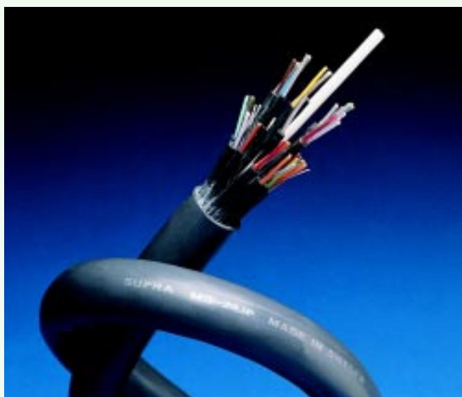
MS20-JP 20 jacketed and screened pairs x 0.22 mm 2 .
