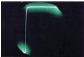
Pict. 1 shows reference with special GR-connected 50 ohm load, acting as a near pure resistance at all frequencies to above 2GHz (high RF).
